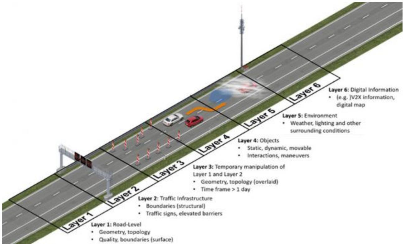
Figure 4.2.: Model for a systematic description of scenarios with six independent Layers DLR (2019)
